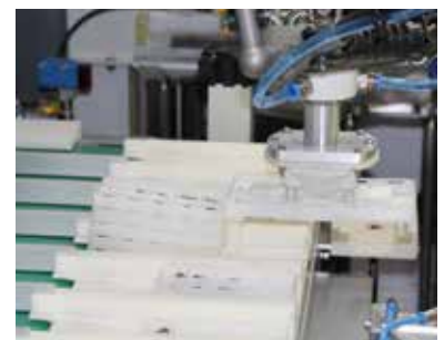
Classification, sorting, tray stacking and ejection on conveyor belt
