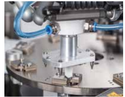
Part handling by 4-axis robot – with vacuum gripper
