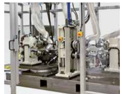
Swivel units and jounce actuator for the simulation of the route
