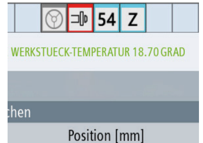
TG82: The temperature is read directly from the control screen
